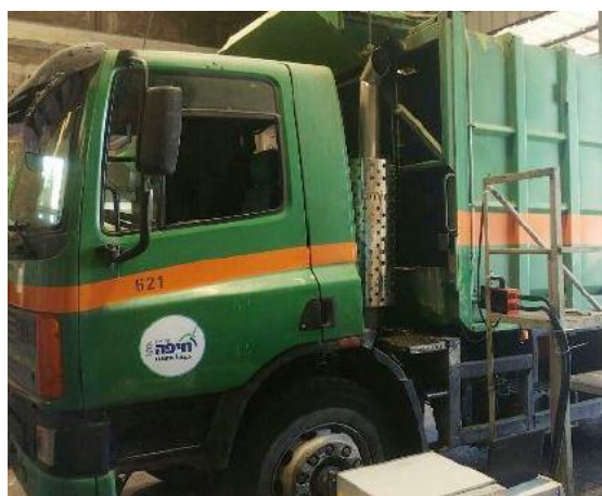
Retrofitted diesel garbage truck
